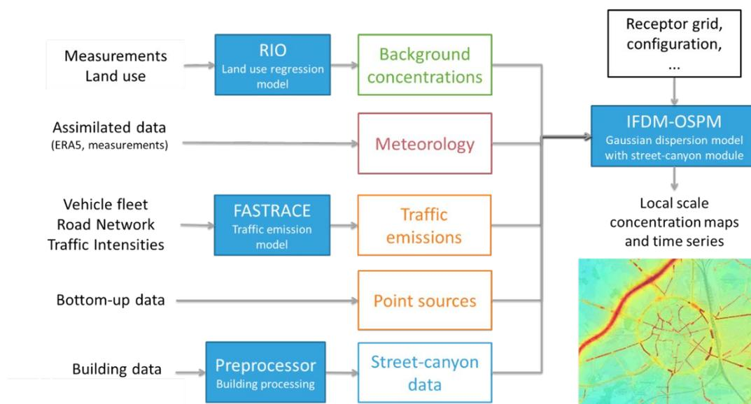
**Figure 1.** Flow chart of the main aspects of the ATMO-Street model.
